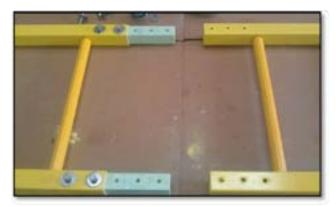
The square tube ladder side rails are produced in 20' lengths so our fab department installed 12" solid square plugs to extend the ladder an additional 5'. We can build ladders and stand-off brackets to any size needed.
