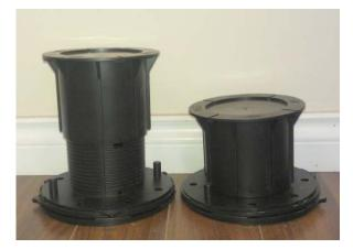
Each V-Series pedestal comes with base slope compensation for up to 1/2" per foot (4%) slope. Simply rotate base pieces for precise slope compensation.
